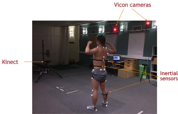
Fig. 6 Static trials. These trials calibrated all streams of data: Vicon and Gait system. Raw data from each sensor was also saved for all trials
