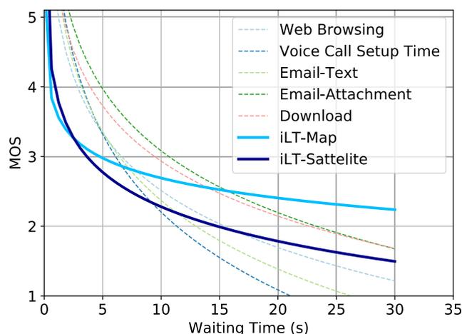
**FIGURE 9.** Comparison between iLT for web mapping application vs State-of-the-Art applications PLT/Waiting Time. The applications can be divided into two categories. The first category involves e-mail transmission with attached files and content downloads. The second category involves the time required to display the home page when accessing a web site (PLT), the time required to connect a voice call, and the time required to transmit a plain-text e-mail [48].
