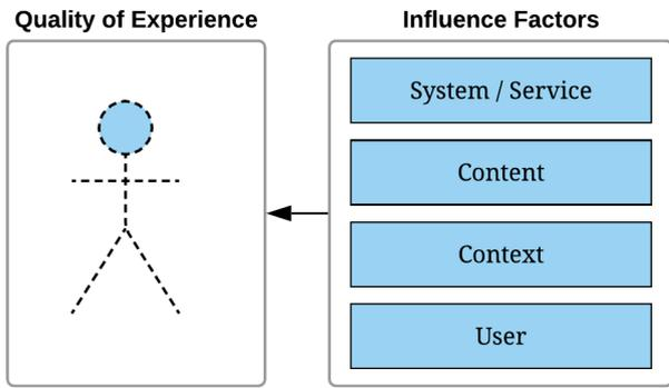
**FIGURE 1.** Illustration of quality of experience influence factors. Considering QoE of Web applications, System/Service factors include the network and computational components, Content refers to how the information is presented (i.e. media type, resolution, content length), Context covers the subject and the theme of the content (i.e. business, leisure, educational). Finally, The User covers the user’s experience and expectations from the web application.
