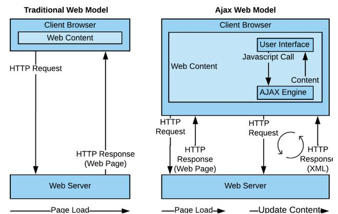
**FIGURE 4. Illustration of traditional web model vs AJAX web model. In traditional web models, an HTML request results in a full page refresh. In an AJAX Web model, the user requests a new content using XHR request and the respective contents/objects will be retrieved and displayed dynamically (an in-place update).**
