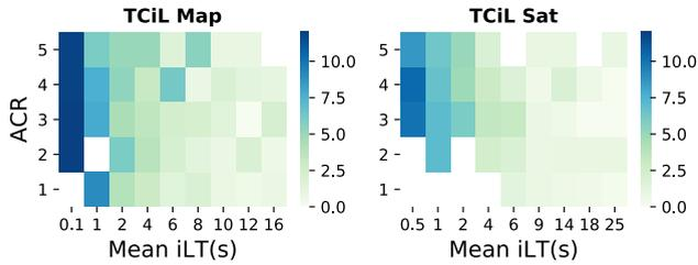
**FIGURE 11.** User behaviour: the relationship between interactive load time (mean iLT) and perceived quality (5 ACR levels) based on the number of completed interactions, TCiLs. The colour corresponds to the number of interactions completed. Plotted by content: map tile (left) and satellite tiles (right).
