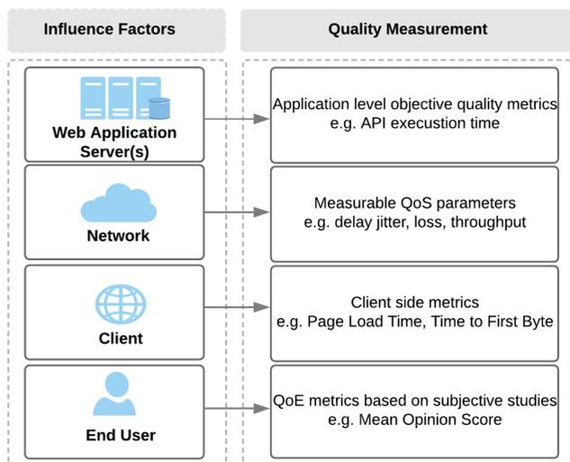
**FIGURE 2.** Illustration of quality measurement in the context of Web QoE. The mapping between quality metrics can help to understand the interdependence between factors.
