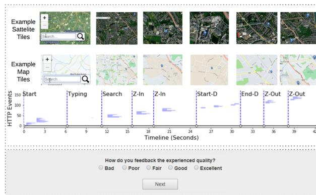
**FIGURE 7.** This graph illustrates an example of the experimental flow and the user’s actions. The x-axis shows the task timeline and the y-axis represents the number of XHR events caused by the user’s interactions. The dotted blue line shows the time that an action is taken and the horizontal blue bars represent the network traffic as a result of user’s interactions. At the end of iteration, the user feedback the perceived quality.
