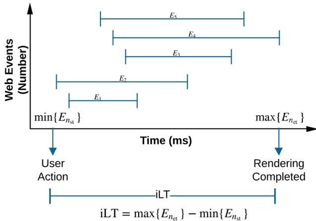
**FIGURE 5.** Illustration of iLT measurement based on the user's interaction and the web events. iLT is measured by computing the duration between starting time of the first event  $E_{n_{st}}$  until the ending time of the last event  $E_{n_{et}}$ .
