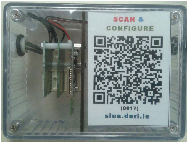
Figure 3. Example for a sensor and its QR code. The QR when scanned returns a URL for the tasks associated with the sensor.
