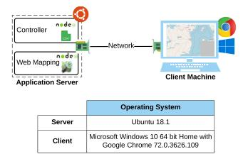
FIGURE 6. The experimental platform developed for the user study. The platform simulated a real network environment and consisted of 2 node servers and a client machine. The network is dynamically manipulated to increase the iLT.
